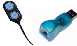
Figure 1: USB connecting cable for iButtons
